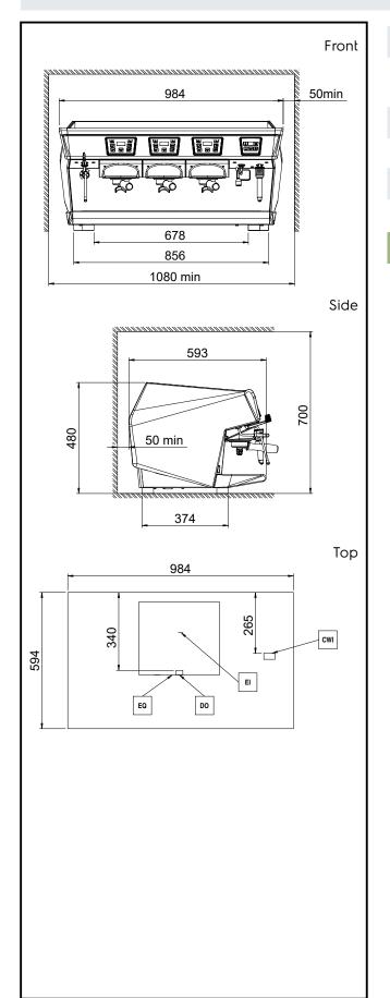
Electric Supply voltage: 400 V/3N ph/50 Hz Electrical power max: 4.8 kW Cable without plug Plug type: Water: Cold water temperature (min/max): 5 / 60 °C **Key Information:** Net weight: 83 kg 0.83 m<sup>3</sup> Shipping volume: Sustainability Current consumption: 7.2 Amps
